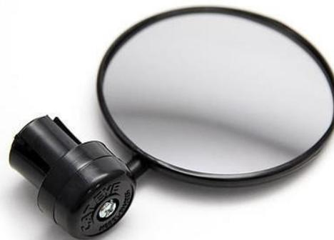
The top example slides over the bar and the bottom one is inserted into the bar and has a bolt that tightens the part that's inside the bar so the mirror doesn't move. Here's a neat trick. If your bike has flat bars instead of the drop bars, to install the bottom type of mirror you'll
