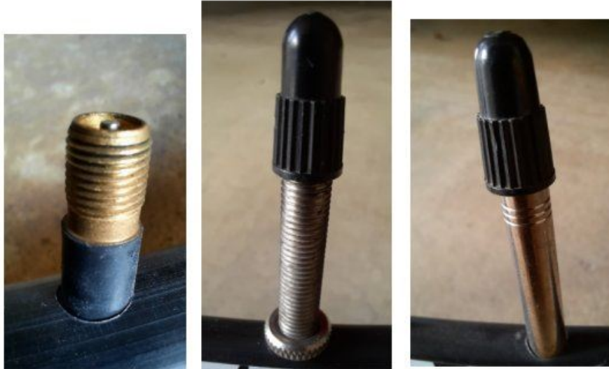
The classic Schrader valve, threaded Presta valve and smooth Presta valve
